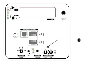
The two DRIVER GAIN switches  $\bullet$  allow the volume of the two horns to be adjusted in –1.5 dB, O dB (= linear) and +1.5 dB steps.
